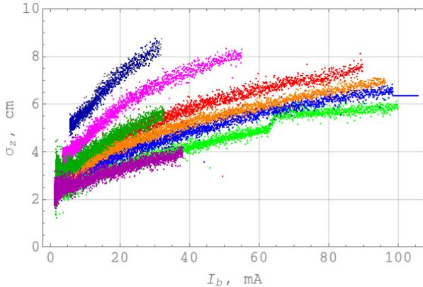
Figure 5: Bunch length at different RF voltages.
