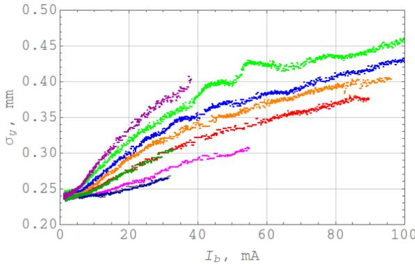
Figure 4: Vertical bunch size at 4MIL.
