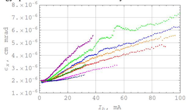
Figure 6: Estimated horizontal emittance for different RF cavity voltages as a function of bunch intensity.
