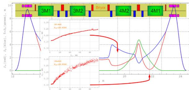
Figure 2: VEPP-2000 lattice functions for the luminosity-taking regime at E=350 MeV.
