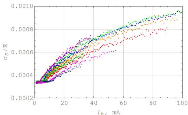
Figure 7: Estimated energy spread for different RF cavity voltages as a function of bunch intensity.
