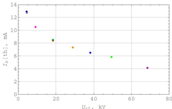
Figure 9: MWI threshold for different RF cavity voltages.
