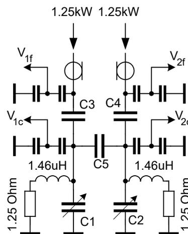
Figure 3: Equivalent schematic of RF cavity/ C1, C2 - 82pF, C3, C4 - 22pF, C5 - 8 pF.
