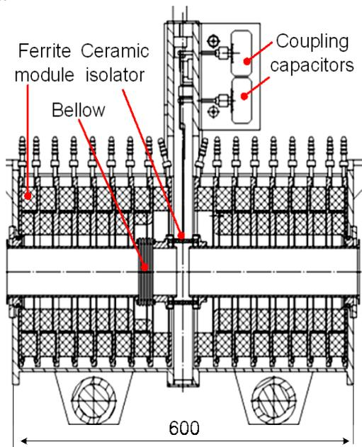
Figure 2: Cross section of RF cavity.
