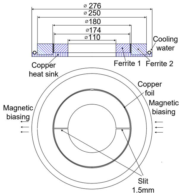
Figure 1: Ferrite module.
