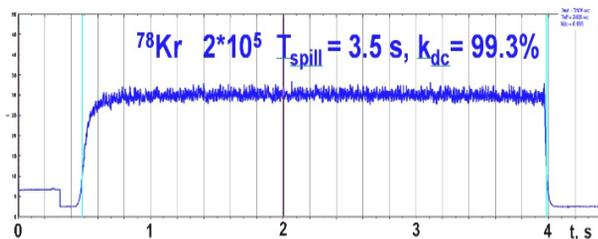
Figure 7:  $^{78}\text{Kr}^{+26}$  beam spill  $2 \times 10^5$  ppp.
