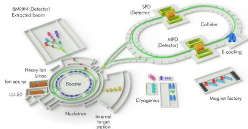
Figure 1: Layout of the NICA Accelerator complex.
