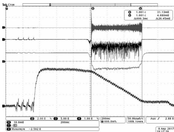
Figure 2: Signals: 1– amplitude of the noise excitation generator, 2 – beam loss monitor M28, 3 - smoothed beam loss monitor M28, 4 – circulating beam intensity.
