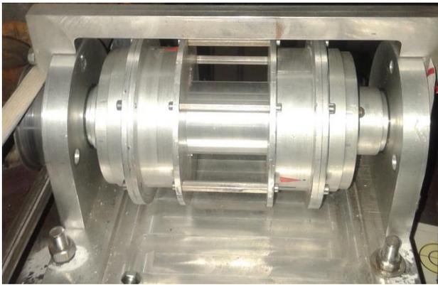
Figure 4: External appearance of mechanical wobbler magnets assembly.
