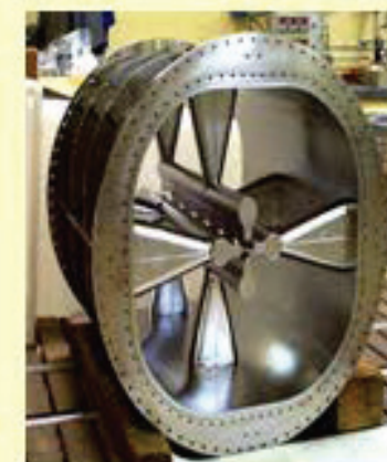
Drift tube with PMQ-lens
