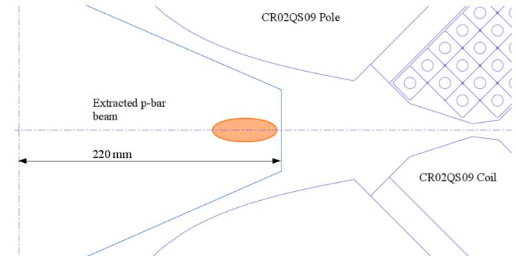
Extracted and injected beams cross-sections @ extraction septum
