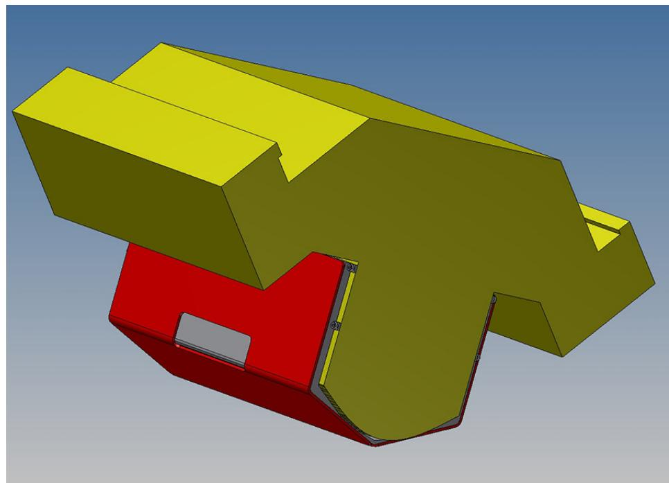
The thin octupole windings are wound in a gap between iron pole and main coil. The quad's pole serves as a support for the octupole winding.
