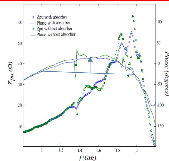
Figure 6: Pickup impedance and nonlinear phase deviation for Faltin rail structure B consisting of two rails of 49 slots each whose signals have been combined. The performance both with and without the presence of ferrite damping material is shown. Simulations are done with a beam centred vertically and with horizontal offset of 40 mm.
