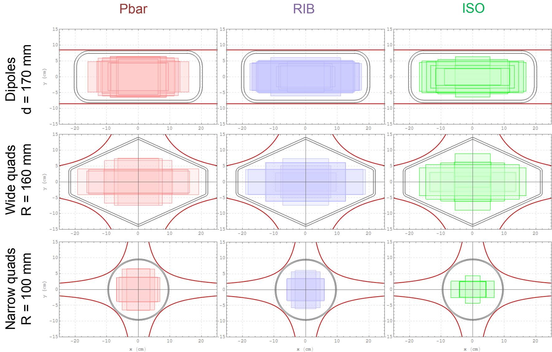
Injected beam cross-sections @ different types of magnets
