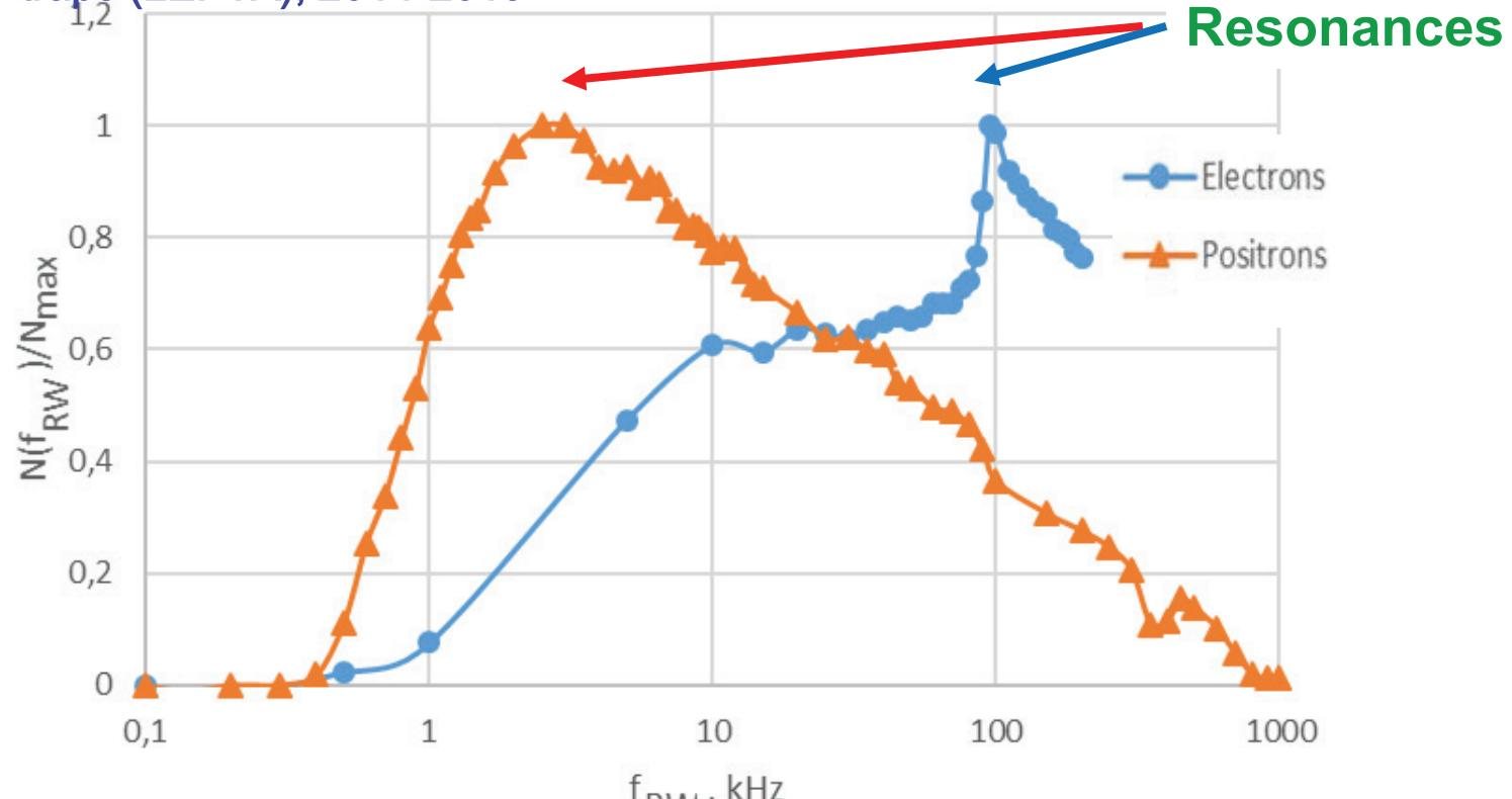
Dependencies of the accumulated electrons and positrons (normalized to the maximum) from the RW-frequency field. The amplitude of the RW-field 1 V, the buffer gas ( $N_2$ ) pressure 2.75 mTorr.
