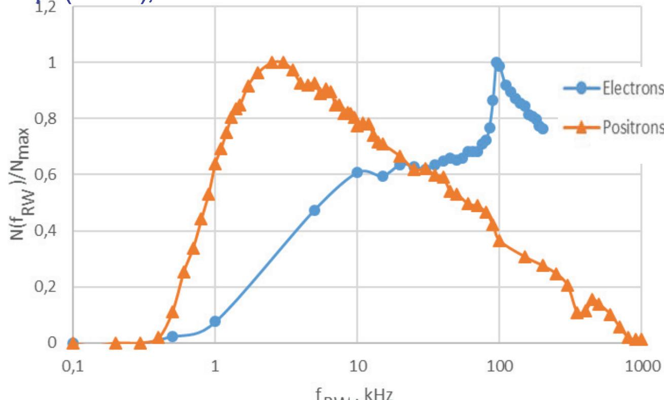
Dependencies of the accumulated electrons and positrons (normalized to the maximum) from the RW-frequency field. The amplitude of the RW-field 1 V, the buffer gas ( $N_2$ ) pressure 2.75 mTorr.
