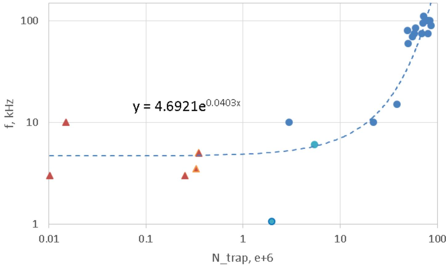
*The particle storage:*  $N_{trap}$ , ( $\omega_{RW}$ ), t=20 s: ● – electrons, ▲ – positrons
