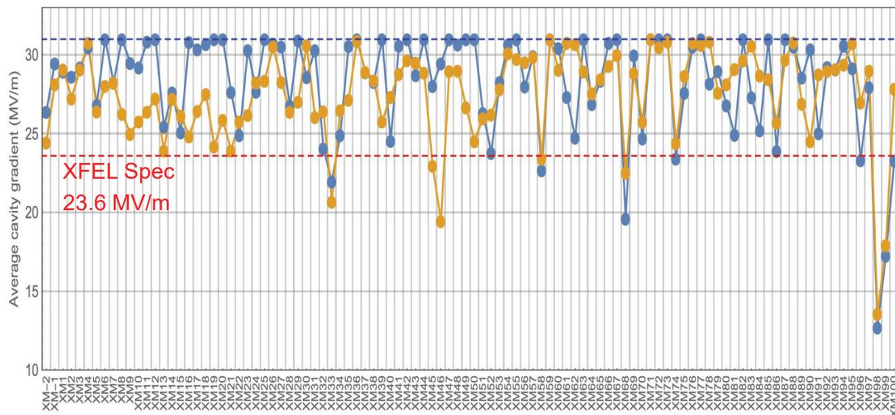
vertical test (clipped at 31 MV/m)
