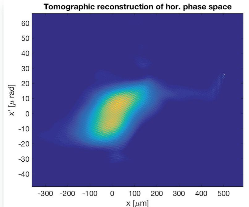
Tomographic reconstruction of the horizontal phase space for the center slice.
