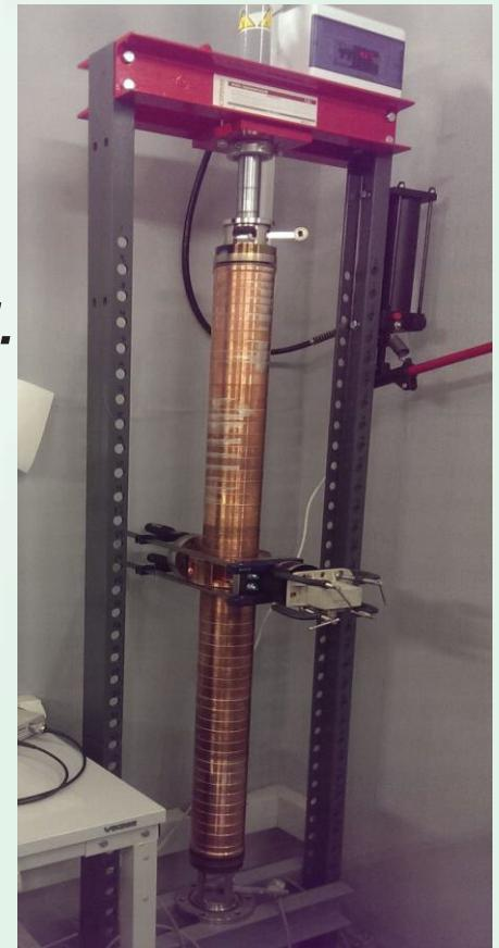
*The first new accelerator was manufactured, assembled and successfully tested at EB Tech Company site in Daejeon, Korea. Control system and some other accelerator components were made by EB Tech. The first accelerated beam was generated on September, 2015. The beam energy was measured by ISO/ASTM 51649:2005(E) Standard.*
