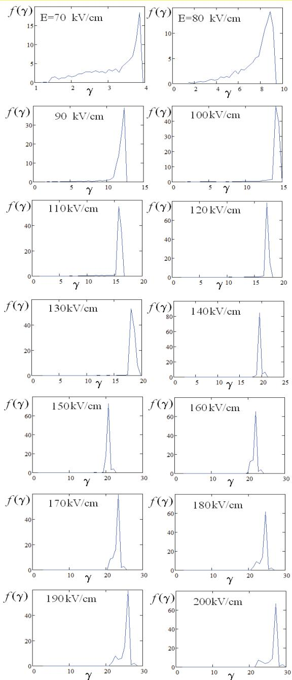
*Output beam energy  $W$  (a), current transmission coefficient  $K_T$  (b) and output energy spectrum measured for full width  $\delta\gamma/\gamma$  on the distribution base (c) vs. injection current for  $E_{max} = 160 \text{ kV/cm}$  and the energy spread measured for total width of the main peak of electron energy distribution vs. RF field amplitude in the range of 70-200 kV/cm.*
