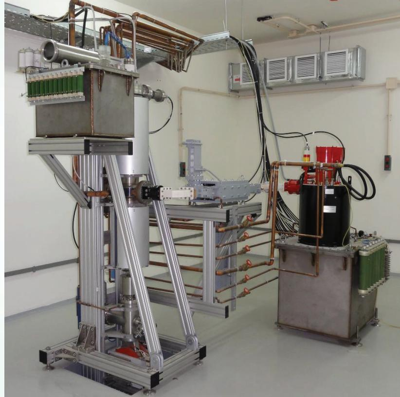
**Since 2005 we made linacs ourselves on the basis of klystron TH2173F but we used accelerating structure made by NIIIEFA**
