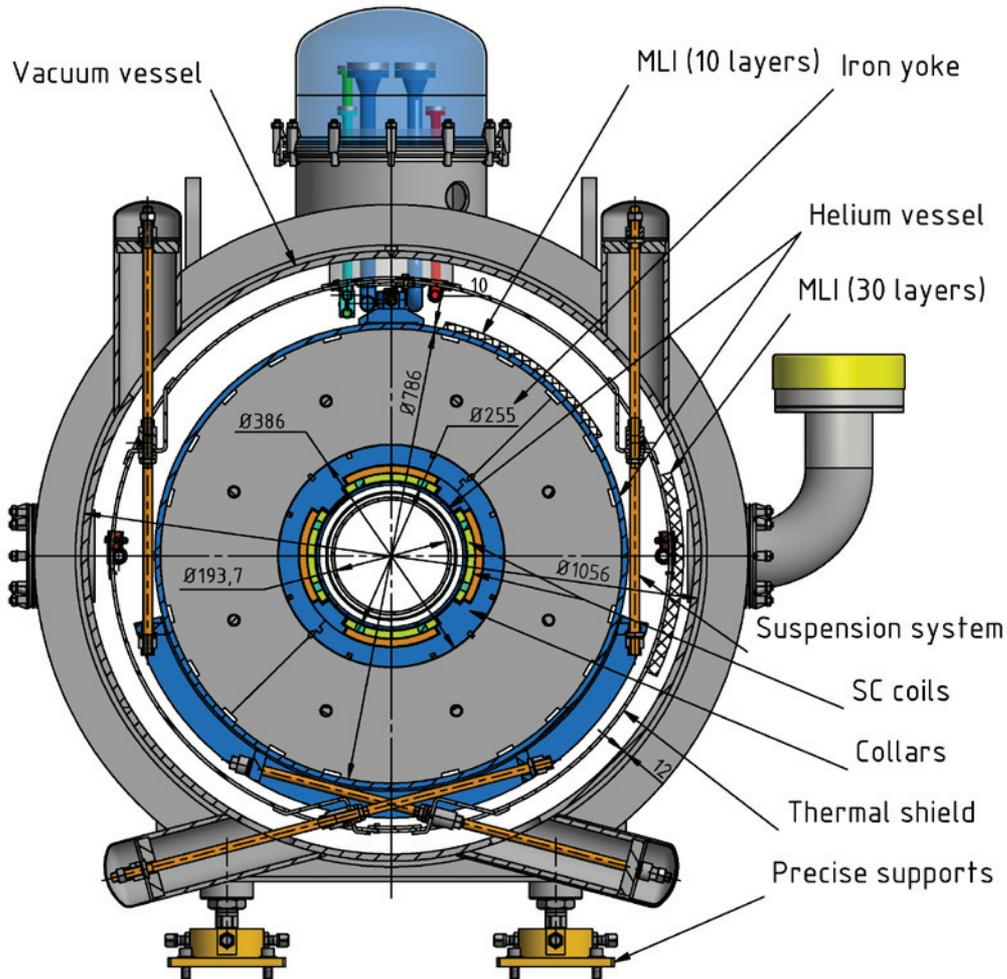
Design of a wide-aperture high gradient quadrupole for final focus system of the HEDgeHOB beam line has been developed.
