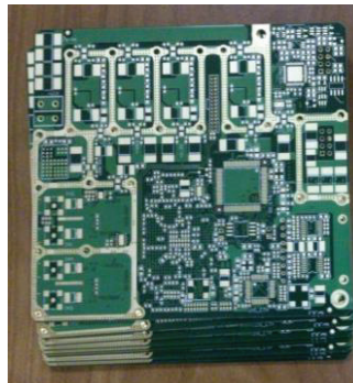
4-channel 200MHz ADC for RF controller
