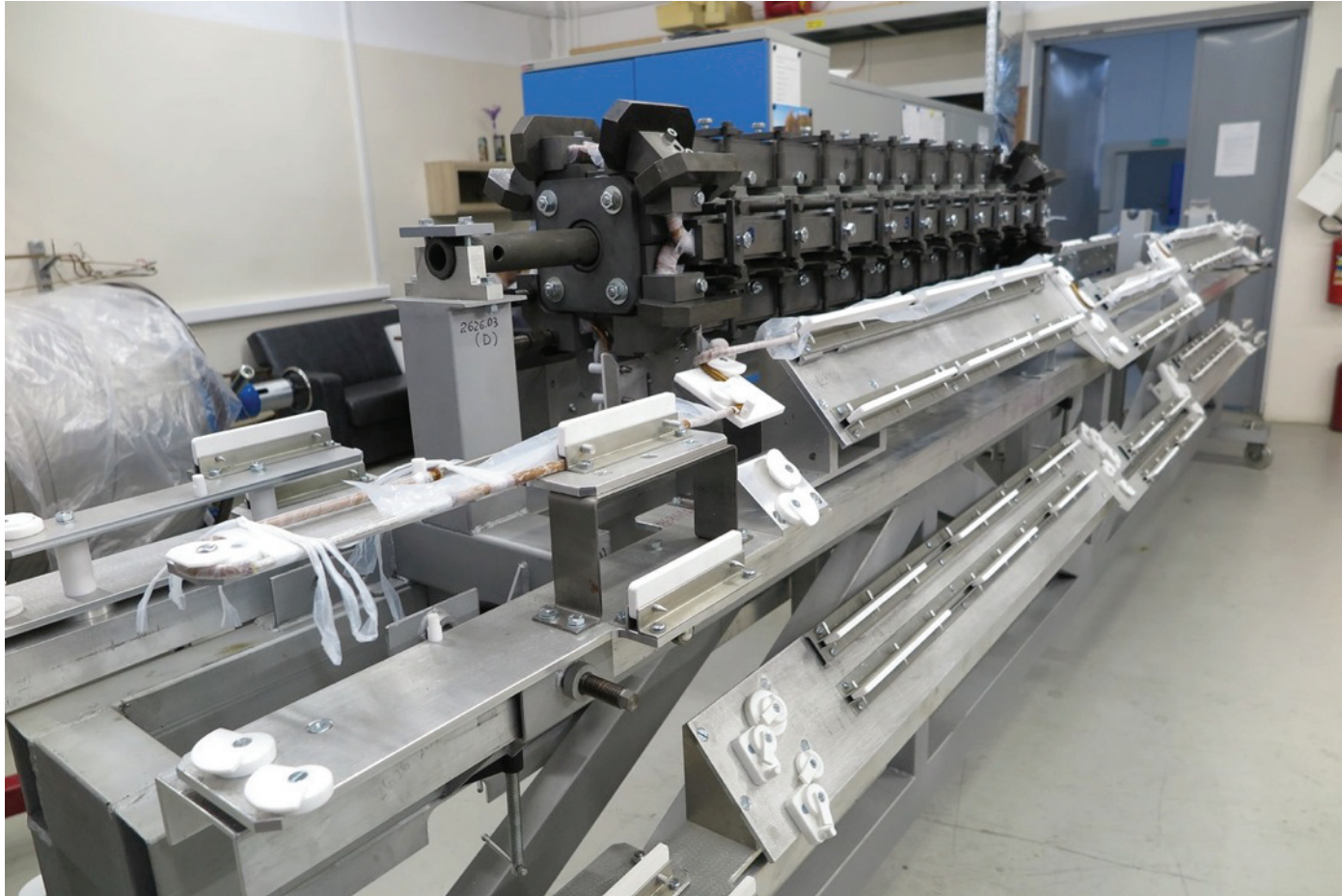
The SIS 100 quadrupole coil prepared for heat treatment in oven
