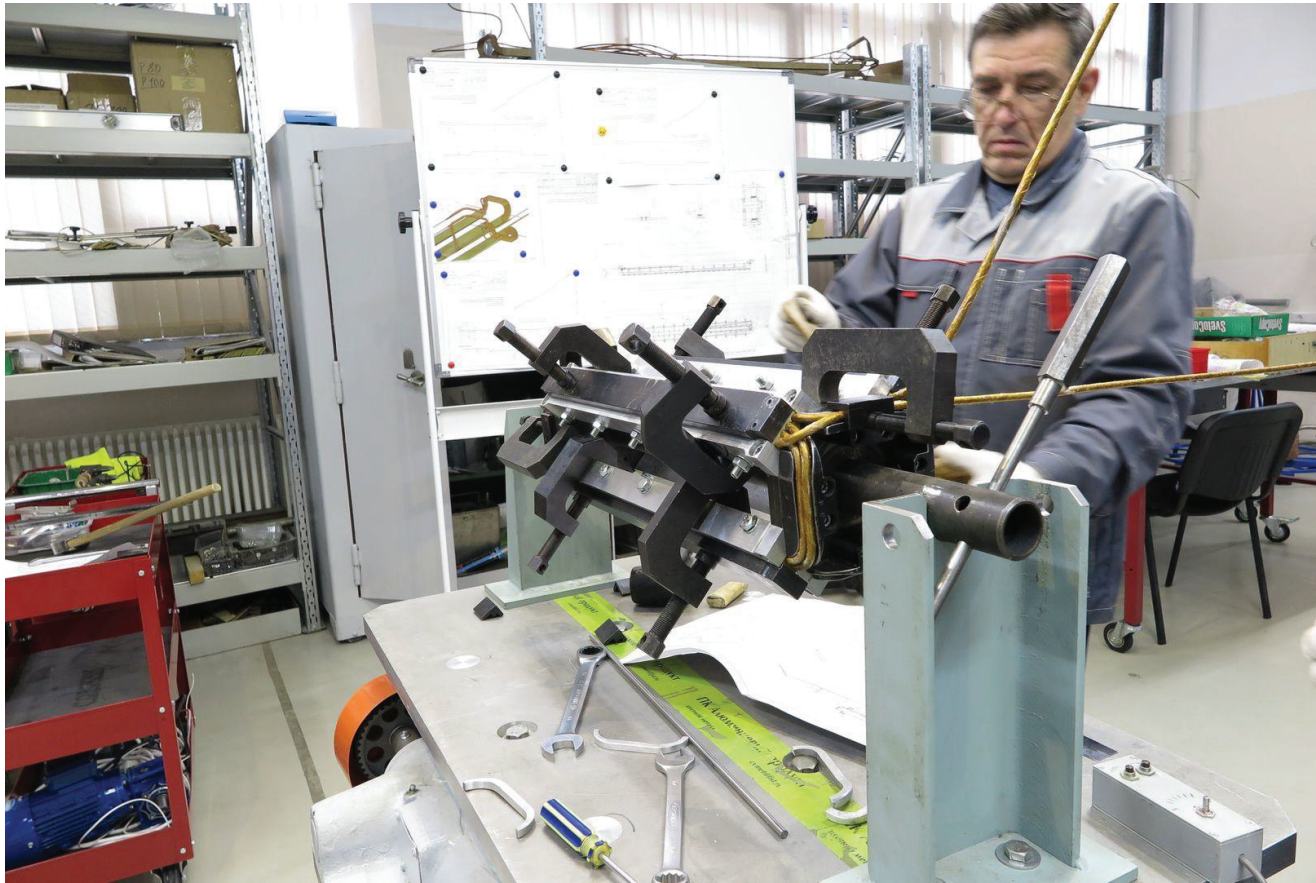
Coil manufacturing for the NICA booster quadrupole magnet
