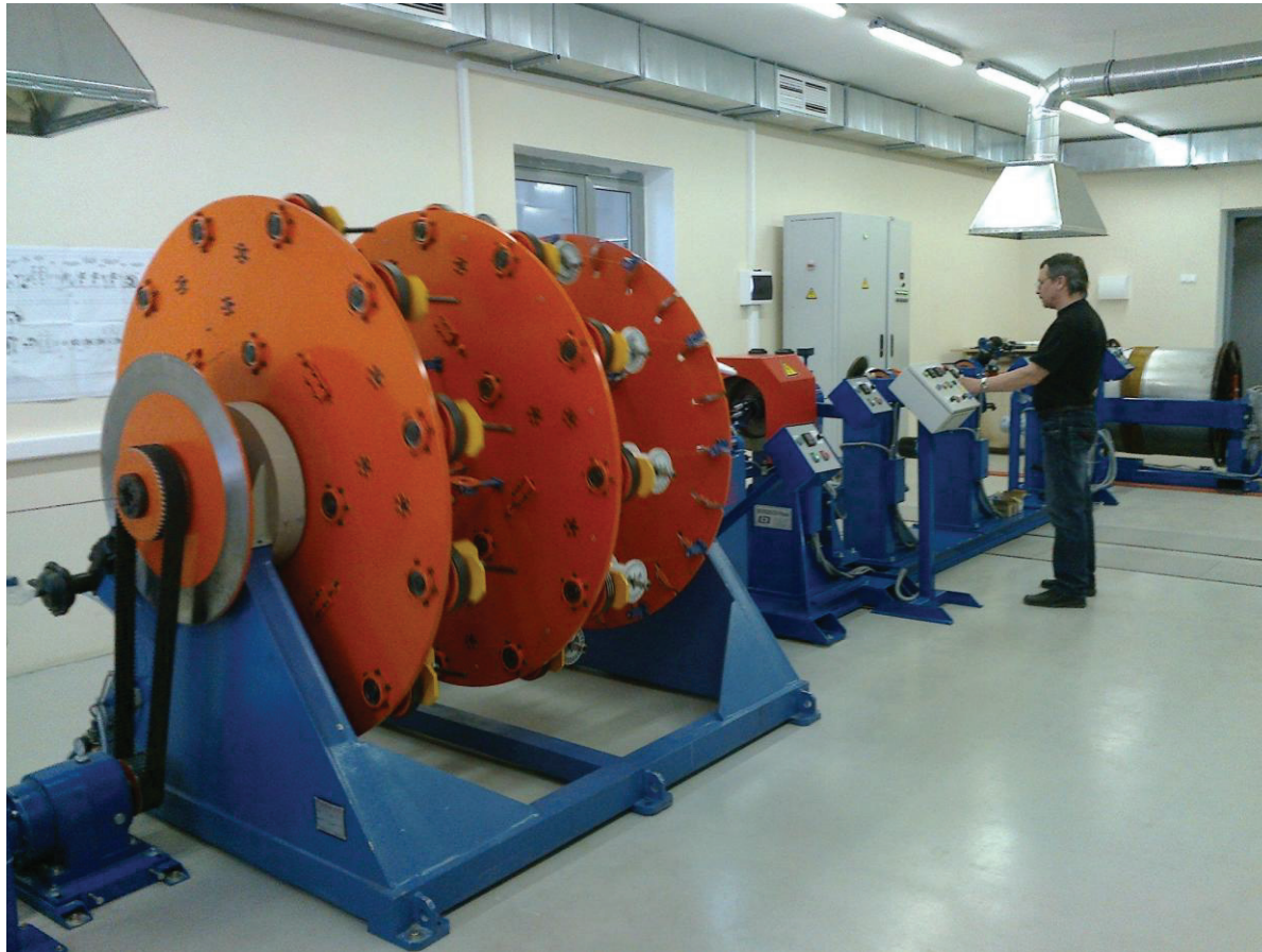
Machine for production Nuclotron-type superconducting cable.
