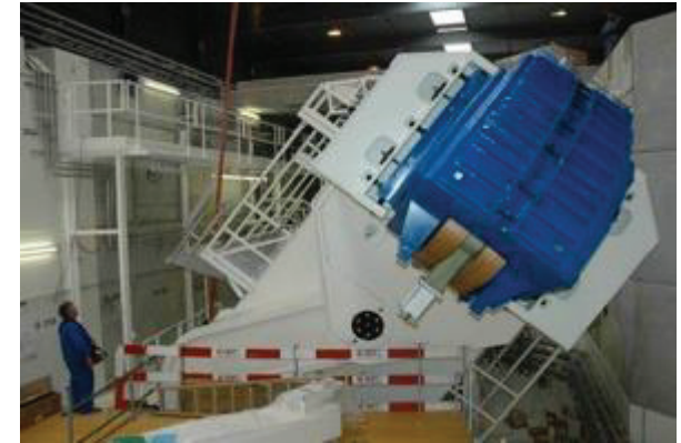
Proton therapy Gantry 2 (PSI) 8m x 12m , 200 tons
