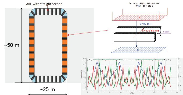
Ring lattice based on QFS concept: ring view with main elements and TWISS functions
