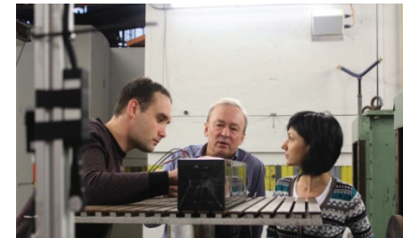
EM calorimeter: Energy resolution = 2.5\% / \sqrt{E}
