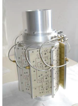
Ring slot-coupler RF structure (design FZJ)
