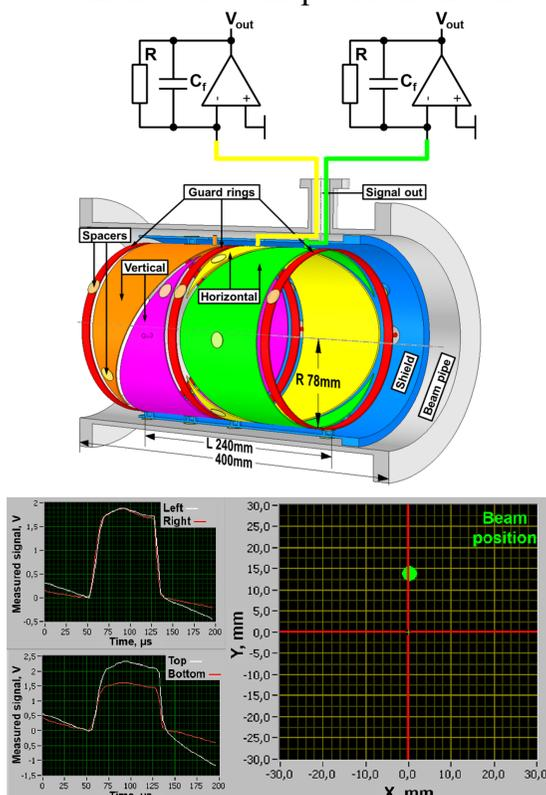
Fig. 3: Pick-up scheme and signals.
