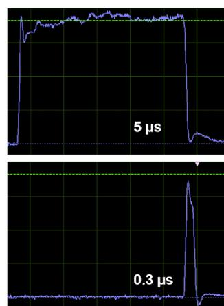
Fig. 4: BCT signals from short-pulse beams.
