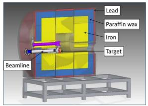
Figure 3: A vertical section along the beam axis through the local radiation shield of the target station.
