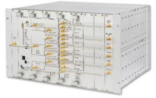
Figure 1: The new digital, low-level RF control system.
