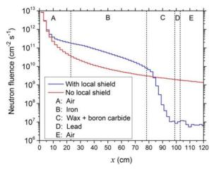
Figure 4: Neutron fluence scan, performed with the FLUKA code, along the x-axis (see text) through the target station for the case of an incident 70 MeV proton beam of 350 µA intensity on a tandem Rb/Ga target.
