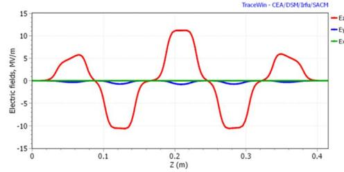
Figure 2: Distributions of the longitudinal and the transverse fields on the axis of the IH-cavity.
