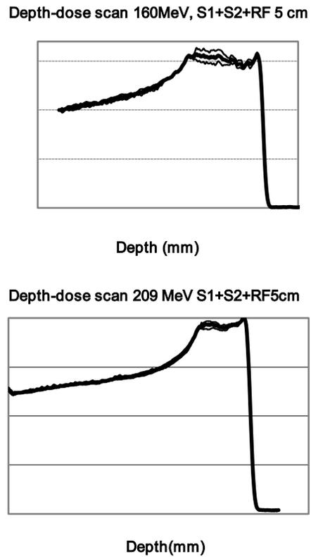
Figures 4 (above) and 5 (bottom): The depth dose distribution for the ridge filters with 5 cm modulation for 160 MeV and for 209 MeV.
