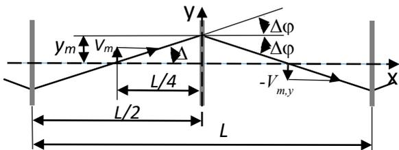
Figure 3: The particle trajectory in the focusing system with short gradient dipoles.
