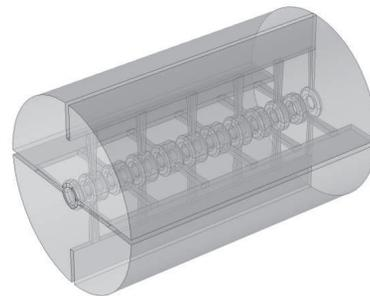
Figure 1: CAD model of the cavity with 11 periods.
