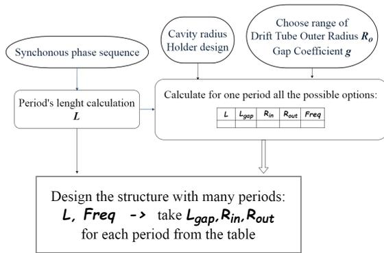
Figure 2: Design algorithm.
