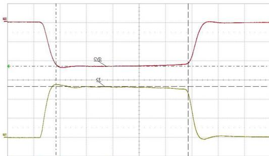
Figure 2: Modulator high voltage (upper trace) and current pulses with amplitudes 50 kV/270 A, respectively. Time scale is 2 μs/div.
