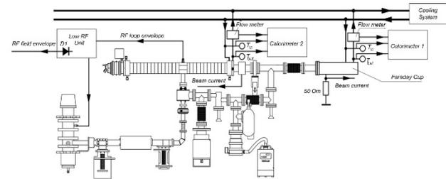
Figure 3: Stand configuration with FC at exit.
