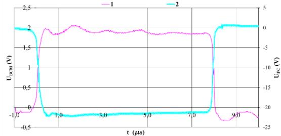
Figure 4: BCT (read curve) and FC (blue) pulses. Time scale is 2 μs/div.
