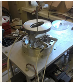
Figure 11: BEP new electrostatic BPM: production (left), test stand (middle), nonlinear calibration (right).
