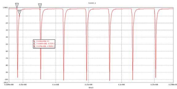
Figure 5: Beam current at the injector output.
