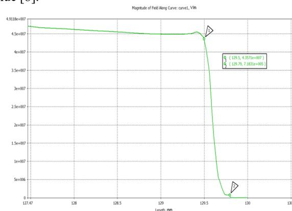
Figure 4: Electric field amplitude distribution penetrating from the accelerating cavities to the cathode-grid gap of the coaxial cavity at the excitation power of 4 MW. Marker 1 corresponds to the cathode position, marker 2 corresponds to that of grid.
