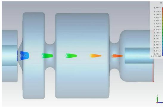
Figure 7: Transverse beam dynamics in the accelerating cavities of the RF controlled RF gun. The bunch is shown in various moments of time.
