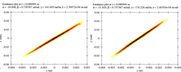
Figure 2: Calculation transverse emittance plot in  $xx'$ -plane (left) and in  $yy'$ -plane (right) from 3D simulation shown in the fig. 1 at  $z=90 \text{ mm}$ .
