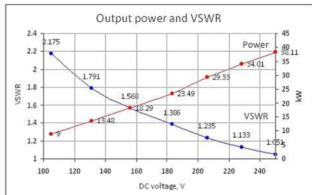
Figure 7: RF power and VSWR vs. DC power voltage.
