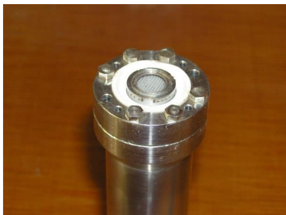
Figure 2: The gun cathode-grid subunit in the assembled condition. The focusing electrode is removed. The outer diameter is 56 mm.
