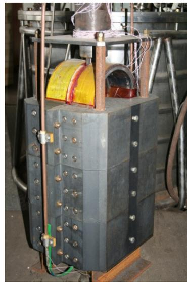
Figure 8: HTS dipole magnet on Bi2223 basis.
