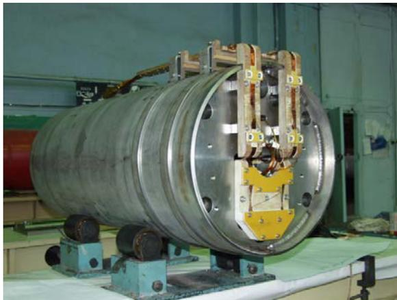
Figure 3: High field fast cycling dipole magnet.
