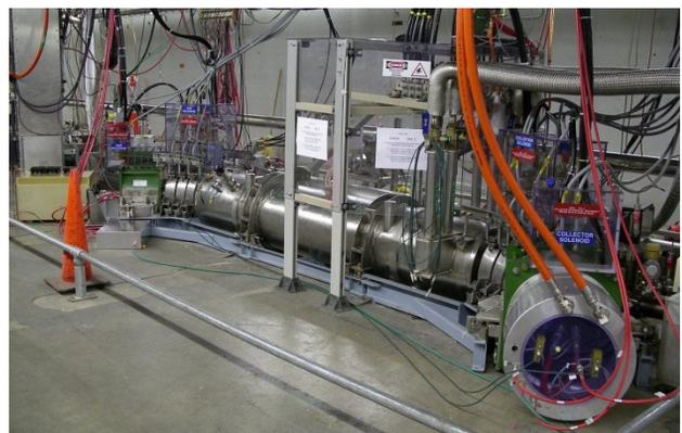
Figure 2: SC magnetic system of Tevatron Electron Lens.
