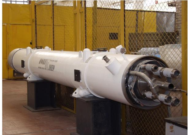
Figure 1: UNK SC dipole magnet.
