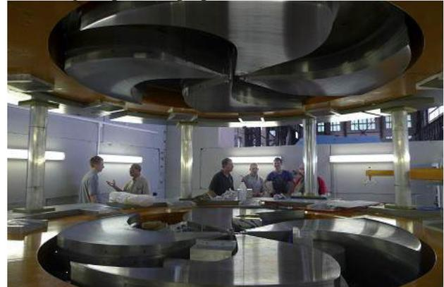
Figure 2: C235 cyclotron in JINR.
