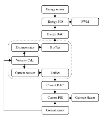
Figure 5: Schematic diagram of stabilization systems.
