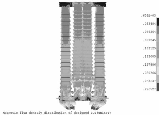
Figure 4: Magnetic flux density distribution.
