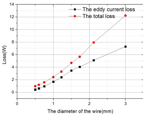
Figure 6: The eddy current loss in different size of the wire.
