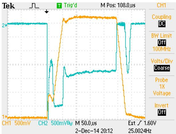
Figure 3: The oscillograms of voltage and discharge current of the H-minus ion source. The top beam (blue) is the voltage at discharge, 50 V/div. The lower beam (yellow) is the discharge current, 10 A/div. Horizontalscale - 50 μs/div.
