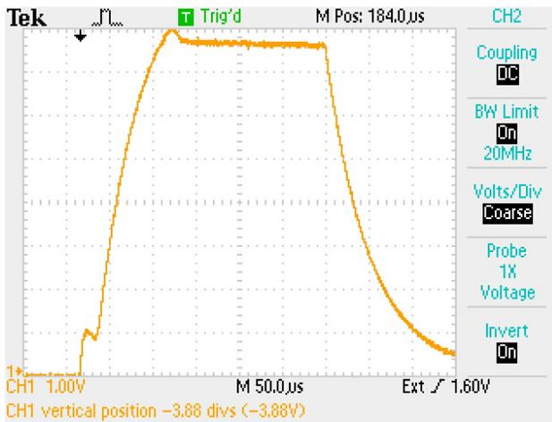
Figure 2: The output current of gas discharge power supplies. Vertical scale – 20 A/div, horizontal scale – 50 μs/div.
