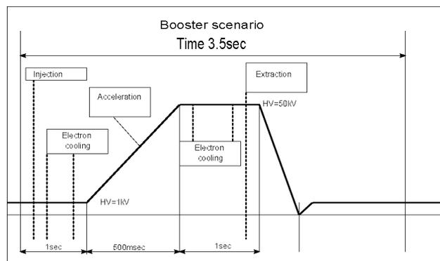
Figure 1: Booster operating cycle scenario.
