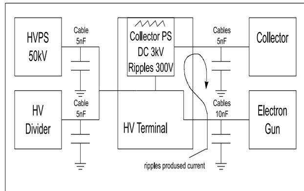
Figure 3. The Cooler high-voltage terminal.
