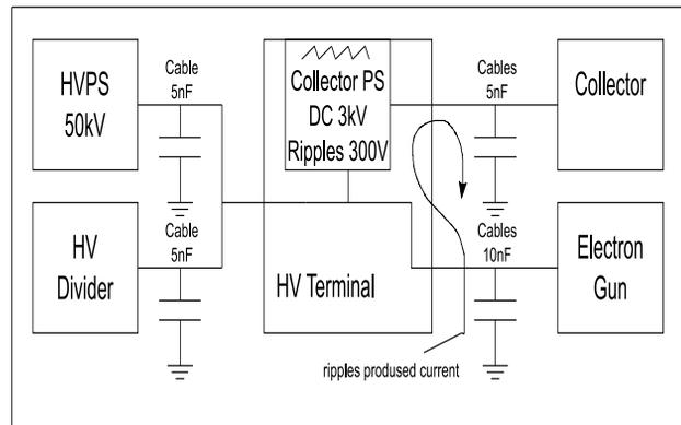
Figure 3. The Cooler high-voltage terminal.
