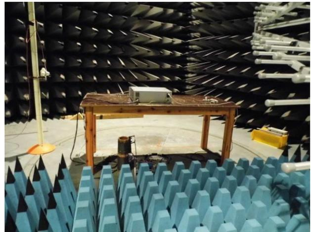
Figure 5: Test set-up for radiated susceptibility.
