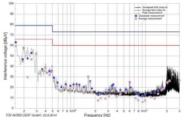
Figure 2: Conducted emission. Disturbing voltage on conductor L.
