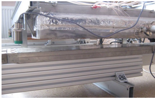
Figure 7: The HTS-II module during tests: maximum levitation gap ~ 40 mm; total current – 14 kAt; total weight of the platform (two HTS blocks with cryostat filled with LN) – 48 kg.
