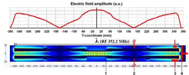
Figure 4: E-field distribution in  $\lambda$ -type deflector.
