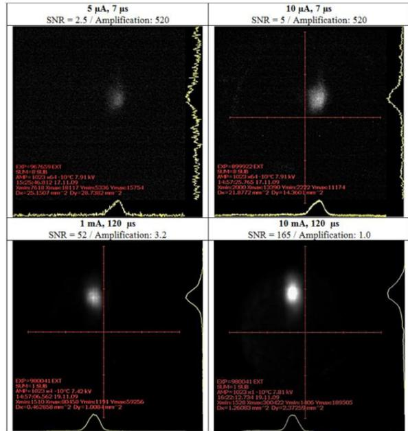
Figure 8: Experimental beam images, registered by BCSM.
