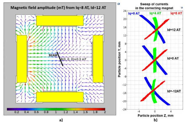
Figure 5: (a) Superposition of dipole and quadrupole fields of the correcting magnet. (b) Cross-sections of the e-beam in the plane of the outlet collimator for different quadrupole Iq and dipole Id coil currents (Ampere·Turns).
