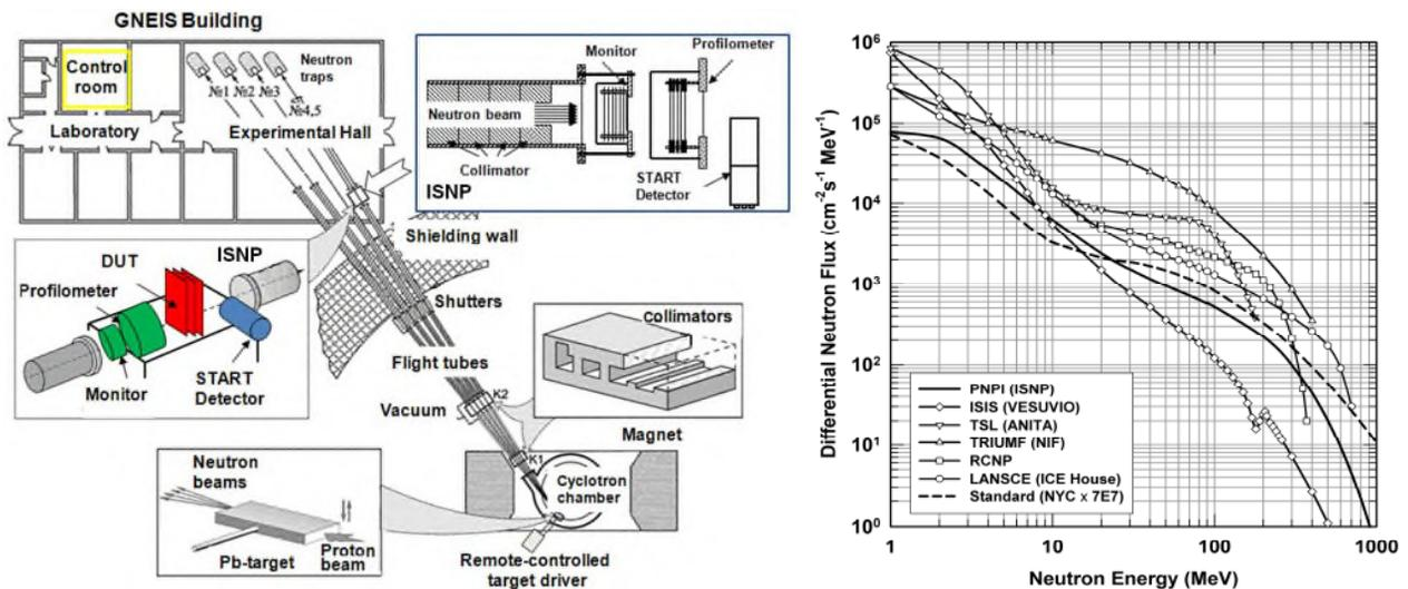
Figure 3: Left: General layout of the neutron time-of-flight spectrometer GNEIS and ISNP test facility. Right: Neutron spectrum  $F_{ISNP}(E)$  of the ISNP/GNEIS facility in comparison with standard terrestrial neutron spectrum and spectra of other world-class test facilities.
