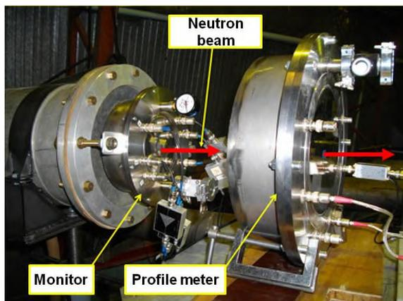
Figure 4: FIC (neutron monitor) and MWPC (profile meter).
