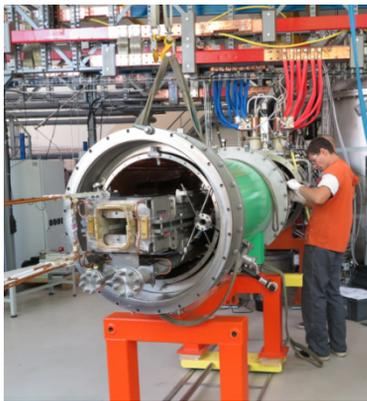
Figure 5: The dipole magnet inside the Booster cryostat.
