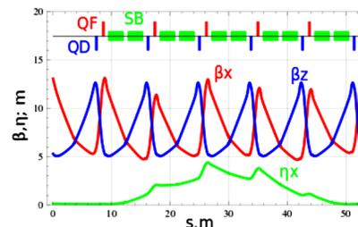
Figure 4: Lattice functions of the Booster synchrotron.
