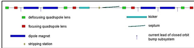
Figure 7: Layout of the beam extraction system.
