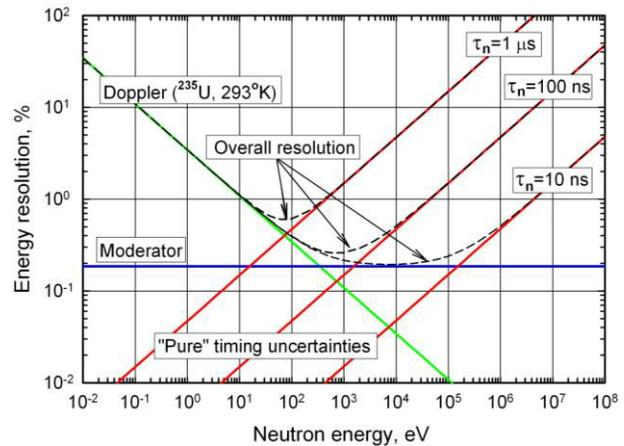
Figure 4: The energy resolution of the GNEIS facility.
