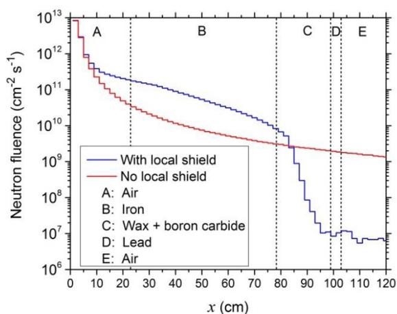
Figure 4: Neutron fluence scan, performed with the FLUKA code, along the x-axis (see text) through the target station for the case of an incident 70 MeV proton beam of 350  $\mu\text{A}$  intensity on a tandem Rb/Ga target.
