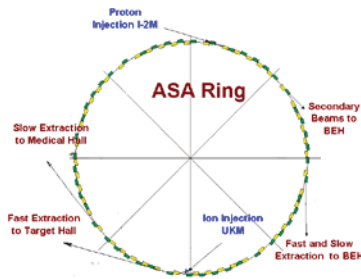
Figure 5: Scheme and parameters of ASA Ring.
