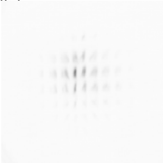
Figure 3: Example photo of the beamlets after "pepper-pot" on the quartz screen.
