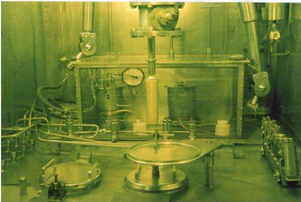
Direct  $^{82}\text{Sr}$  sorption from liquid metallic rubidium containing oxygen (0.1 – 4 wt.%)
