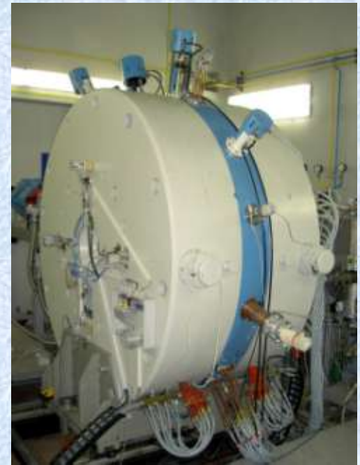
The CC-18/9 Cyclotron in the PET center, Chelyabinsk region, Russia. Delivered in 2010.
