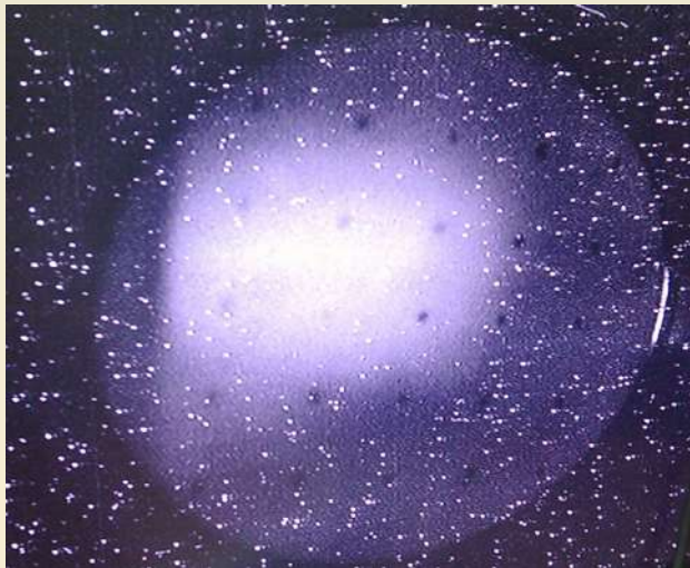
Electron beam on phosphor screen after the tenth acceleration section
