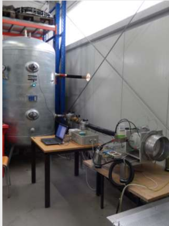
Pressure tank and turbine
