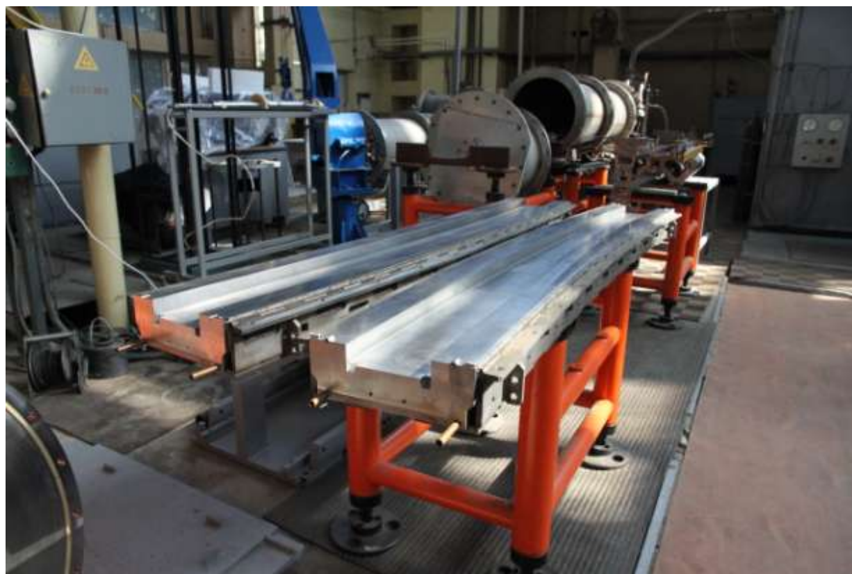
Half-yokes of the NICA Booster dipole
