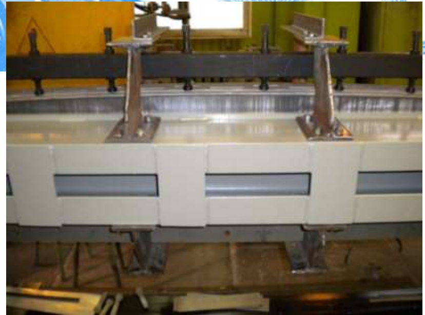
Assembly of iron plates, compression in axial direction with 50kN
