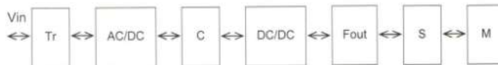
Figure 2 Block diagram of the supply with recuperation to the supply network
