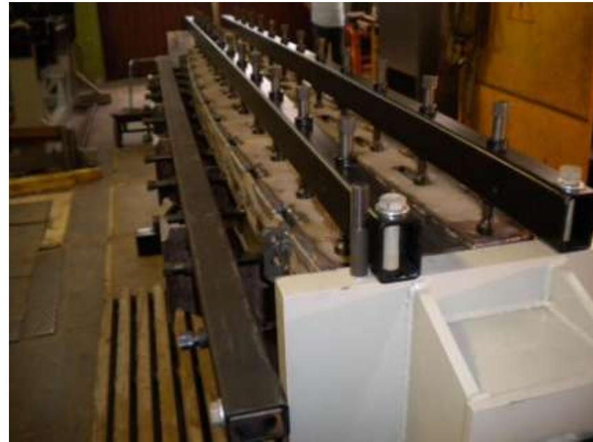
Assembly of iron plates, compression in axial direction with 50kN
