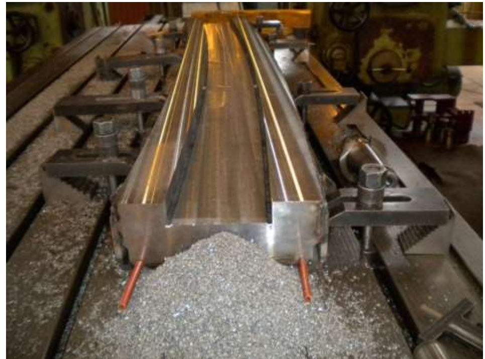
Final machining of half of the yoke
