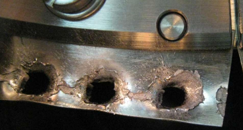
Target explosion due to electron beam energy deposition generates tantalum drops with very high velocity (up to few km/s). These drops damage the emission ability of the cathode and reduce the electric breakdown strength of diode and further accelerating tube electrodes. This is why LIA-2 can reliably operate 2 MeV, 2 kA without target explosion and only 1.6 MeV, 1.5 kA with target explosion.
