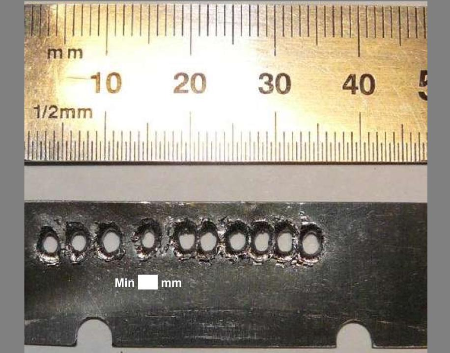
For fixed beam energy and current the hole diameter in the target can be changed by final lens strength regulation (from minimum possible to maximum possible value).
