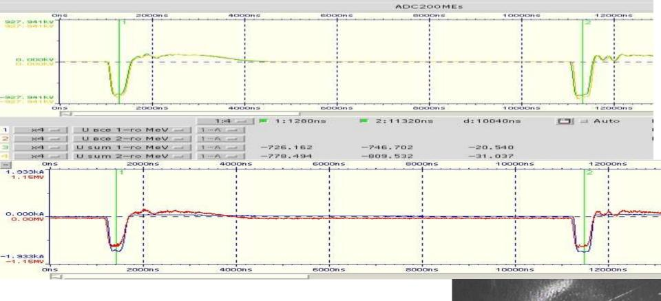
Two pulse operation of LIA-2, 1 mm thick Ta target. 1.6 MeV, 1.5 kA.
